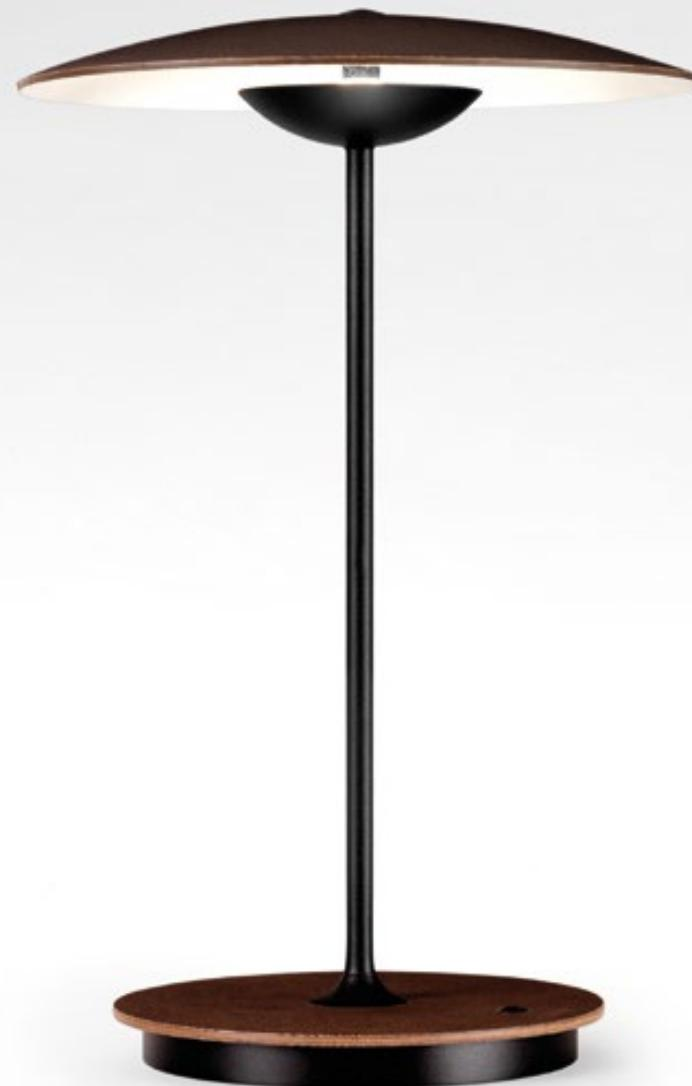
**Diffuser and pressed wood base of 4 mm in natural oak or wenge. Injected aluminium dissipater and lacquered black matte metal stem. Battery is located inside the base, with 5 hours of battery life at peak performance.**
