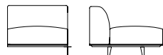
*SF 65002 C Elemento centrale rivestimento tessuto o pelle Central element fabric or leather upholstery cm 83 x 100 x h 68 in 32 5/8 x 39 3/8 x h 26 3/4
