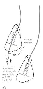
Thread the coaxial cable through the shade, followed by the trumpet and finally slide on the trumpet retainer.
