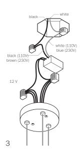
Connect the coaxial cable to the open slots in the terminal block on the 12V side of the transformer. Ensure that the braided outer wires are all connected to one 12V output wire and all inner insulated wires are connected to the other or a short will occur.
