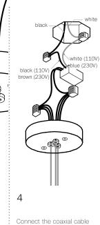
Connect the coaxial cable to the open slots in the terminal block on the 12V side of the transformers. Ensure that the braided outer wires are all connected to one 12V output wire and all inner insulated wires are connected to the other or a short will occur.
